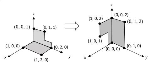
3. An object is to be reflected about a plane passing through the point (3, 0, 0) as shown in the figure below. The reflection transform is obtained with a series of basic transforms. State the series of transformations required and the transformation matrix for each of these basic transforms. (12 marks)
